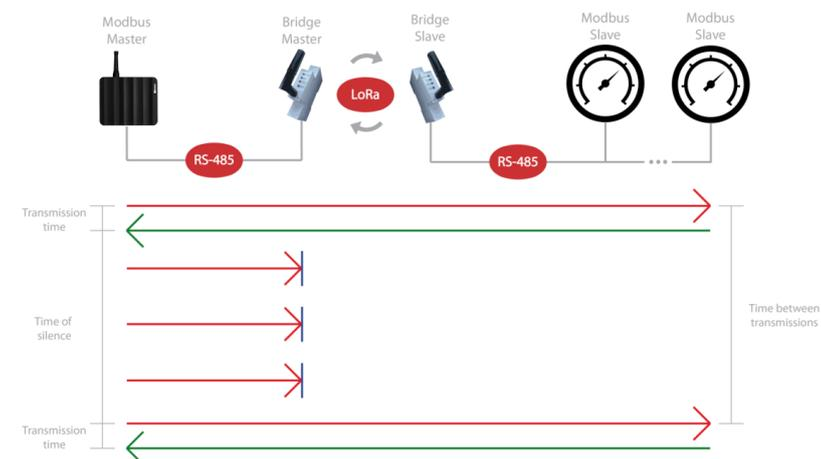
Based on these times, 2 communication rules are established that must be applied in the Master Modbus of the installation. The first one, described below, is absolutely essential to establish wireless communication with the Modbus slaves through an SBL8 wireless network:
