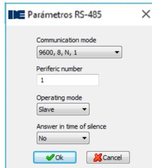
By accessing we can configure the parameters Communication mode, Peripheral number, Operating mode and Response in silence time. The mode will allow us to select if the SBL8 that we are configuring will be the Master of the installation or Slave. If 'Response in silence time' is enabled, the Master SBL8 will respond 'Busy' through the Modbus line if it is found during the silence time, while if it remains disabled it will not send new transmissions
