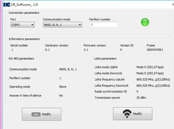
For the parameterization of SBL8 is required a PC software that can be downloaded free of charge from the website [www.disibeint.com](http://www.disibeint.com).
