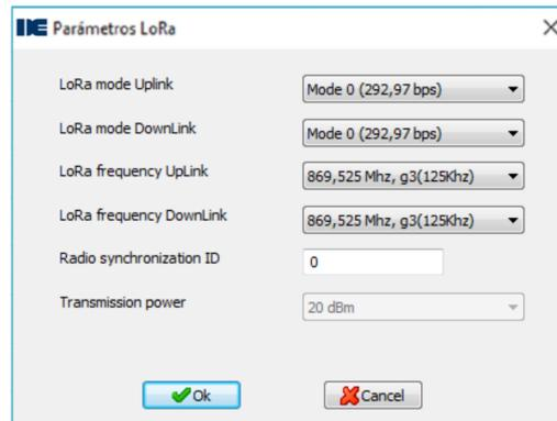
By accessing we can configure the parameters LoRa Uplink Mode, LoRa DownLink Mode, LoRa Uplink Frequency, LoRa DownLink Frequency, LoRa gateway ID, transmission power and radio synchronization ID.
